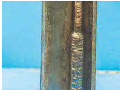
Multi pass welding - vertical up
