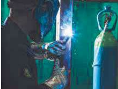
MAG welding of carbon steel
