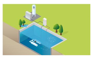
On top of its robust design, the **OXY INJECTOR-VENTOXAL** is both compact and easy to use. The standard version consists of frame, pump, gas-liquid nozzles and mixing unit. The largest unit can inject up to 240 kg/h of oxygen. Multiple **OXY INJECTOR-VENTOXAL** systems can be easily combined to meet the need for dissolved oxygen in the basin.
