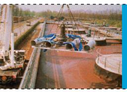
Oxygen can be added by several gas/liquid transfer devices including VENTOXAL.
